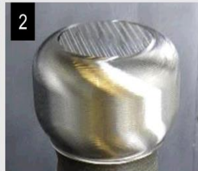
2 Milling of the basic body
