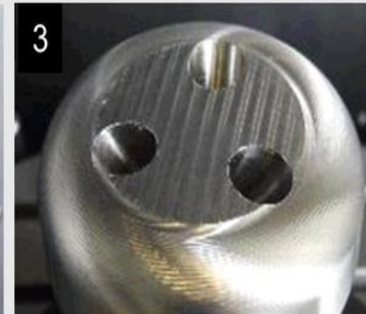
3 Drilling of coolant holes
