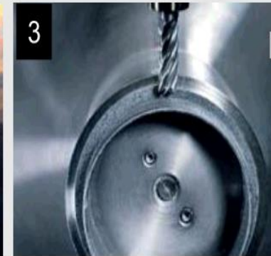
3 Milling of the flat and the perimeter
