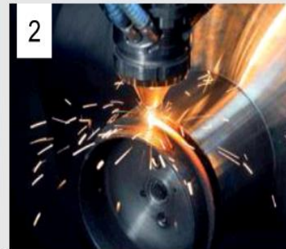
2 Swivel to 90°: Generating of flange
